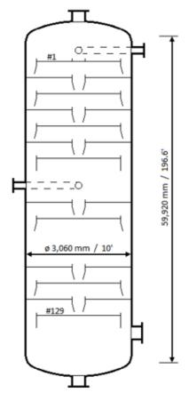
Fig. 13: Grass root design of a Butane Splitter with Raschig's to high capacity Mini Fixed Valves
