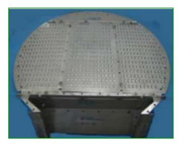
Fig 12: Tray deck layout applied for revamp project with Raschig Mini Fixed Valves and downcomer adapters
