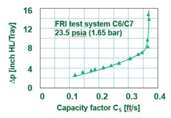
Fig. 5: Pressure drop and capacity over column cross section area related Cs-factor of Raschig Mini Fixed Valves tested at FRI with cyclohexene/n-heptane at 1.62 bar (24 psia)
