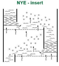
Fig. 14: Principle flow scheme of a NYE insert
