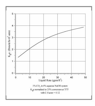
Low Profile Rings have significantly higher masstransfer efficiency than conventional packings.
