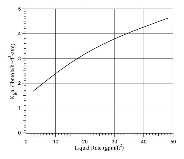
$1\% \text{ CO}_2$  in 4% aqueous NaOH system  $K_g$ a normalized to 25% conversion at  $75^{\circ}$ F with C-Factor = 0.12
